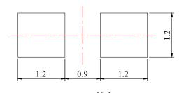
Unit: mm Tolerance: ±0.10mm
