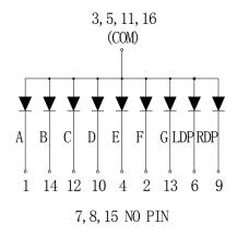
Internal Circuit Diagram (Common Cathode)
