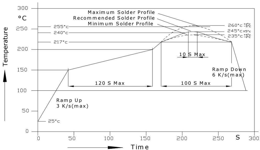
1.11. Reflow soldering should not be done more than two times.
