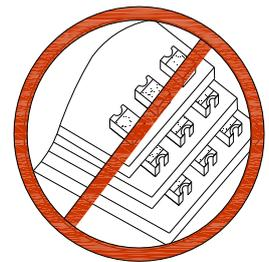
Compare to epoxy encapsulant that is hard and brittle, silicone is softer and flexible. Although its characteristic significantly reduces thermal stress, it is more susceptible to damage by external mechanical force. As a result, special handling precautions need to be observed during assembly using silicone encapsulated LED products. Failure to comply might lead to damage and premature failure of the LED.
