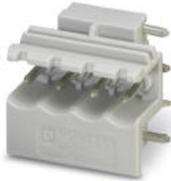
Header, Nominal current: 12 A, Rated voltage (III/2): 320 V, Number of positions: 4, Pitch: 5 mm, Assembly: Soldering
