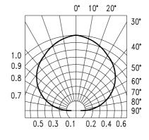
Fig.5 Luminous Intensity vs.
